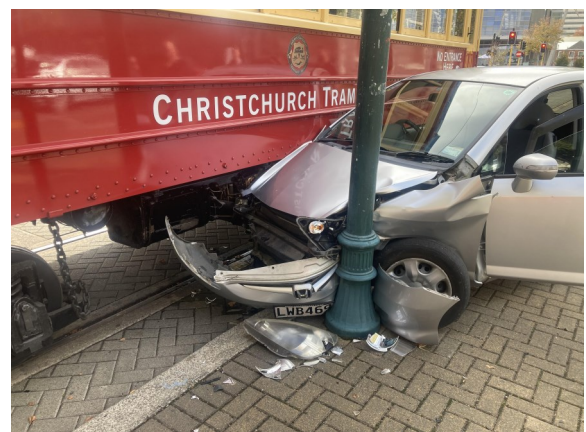
178 with the car wedged between the PC5 controller and a traction pole at stop 12.
