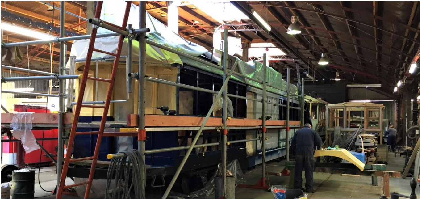
ABOVE: As described on p.6, Restaurant Tram 411 has been turned around for the completion of its overhaul in Tram Barn 1. With Brian Fairbrass at right working on 411's end canopy apron and windscreen, Dave Hinman captured 411 together with glimpses in the background of the Christchurch No. 24 and Mornington No. 103 restoration projects. Photo: Dave Hinman.
