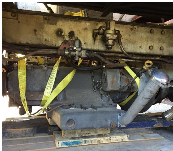
410's motor back under the bus, sitting on the pallet and temporarily tied. (Photos: D Hinman)
