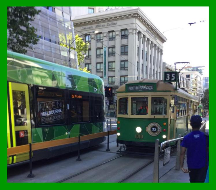
**ABOVE:** Old meets new during the morning peak hour. Not yet in service for the day, 1955-built W8-class tram 1010 — one of six W-series trams rebuilt in Bendigo since 2013 for use on Route 35 City Circle duties—passes its modern-day equivalent, 2016-built E-class tram 6047 outside Southern Cross Station. 02/02/2018. Photo: Alastair Cross.
