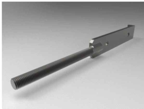
Model of existing chassis wrought iron anchoring bolt
