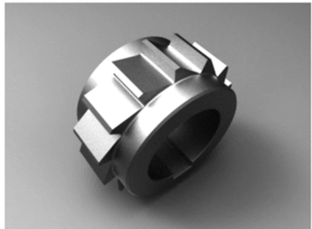
Runback pawl modelled from Dunedin Tramways Drawings
