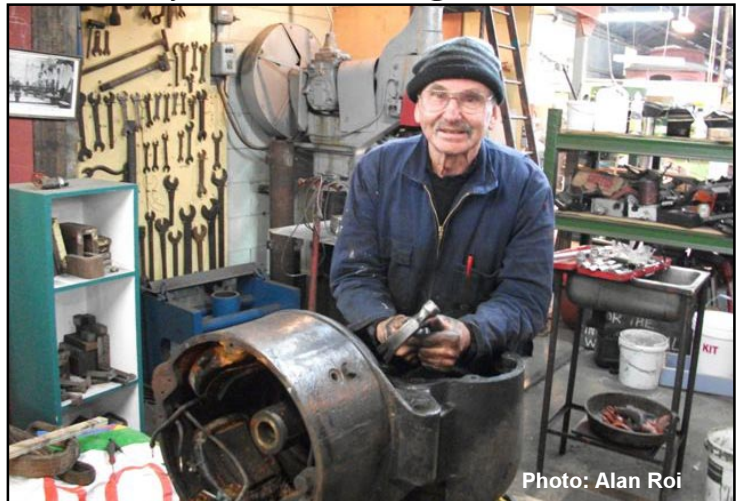
Murray Sanders at work restoring the compressor for Hills car No 24.
