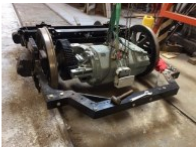
BOTTOM RIGHT: Both a compressor and a compressor governor (not shown) have been overhauled ready for fitting. Photo: Dave Hinman.
