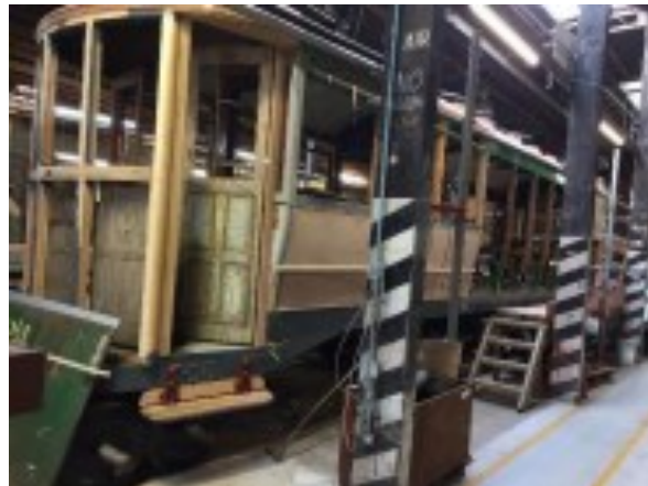
ABOVE LEFT: The seat bases at the bottom of the open section pillars have been refitted again after painting Photo: Stephen Taylor
